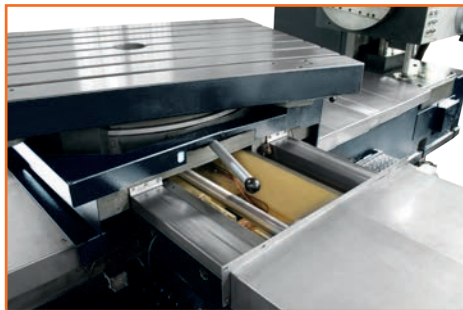
Gear drive of the swivel work table mechanism (below)
