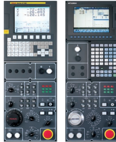
Fanuc Oi-MD (left) and optional Mitsubishi CNC control (right)
